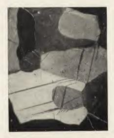
Fig. 15. (x 30 Diameters. Oblique Illumination.) Base of Small Ingot of Zinc Cast on Stone.
